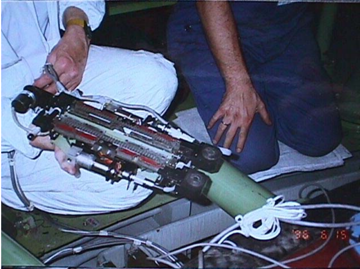
Figure 11. Robotic Inspection Vehicle – Covers removed
