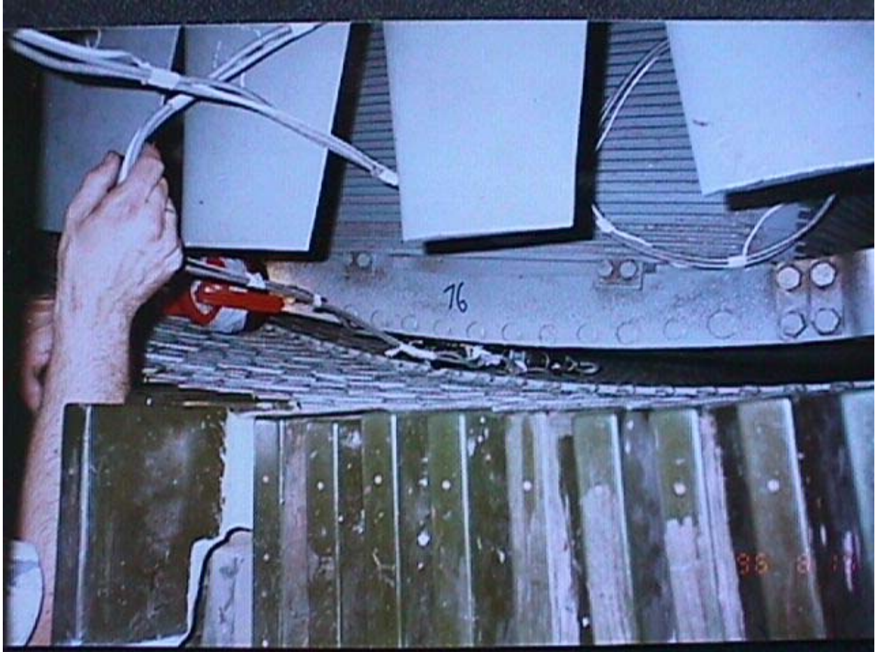
Figure 12. Robotic Vehicle in place to scan a single slot
